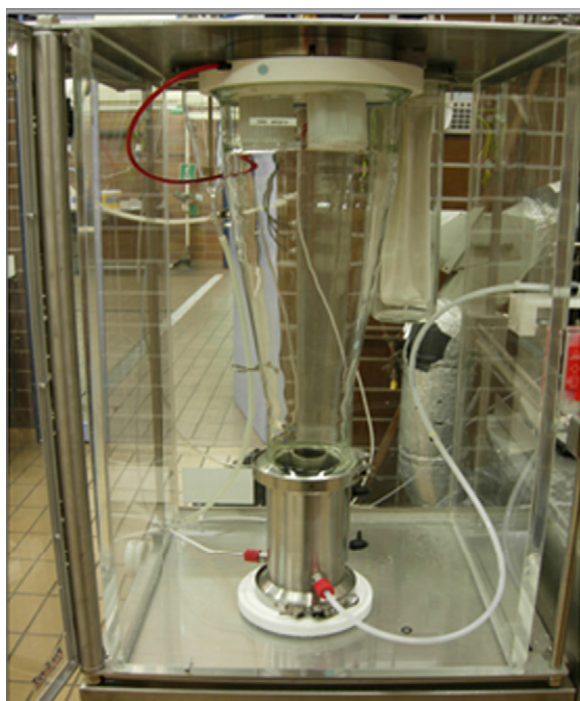
Fig. 4. Laboratory re-circulatory fluidized bed granulator (System B).
